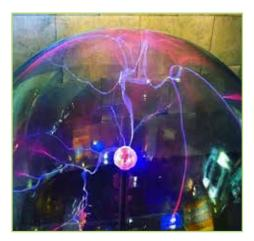
The glass is filled with a mixture of various noble gases, commonly neon, argon, xenon, or krypton. A very high voltage is created by a Tesla coil-like circuit setting up a high electric field between a central electrode and the inner glass. The electrode at the center of the plasma ball emits a high-frequency, high-voltage alternating electrical current. This current flows through the plasma filaments to create colorful tendrils of light. The color depends on the gases used.
